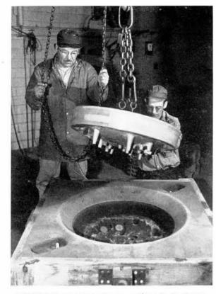
A MOLD is necessary for a casting. C. B. Torres, left, and Donald Quayle have made the mold in damp sand and are shown here removing the pattern.
